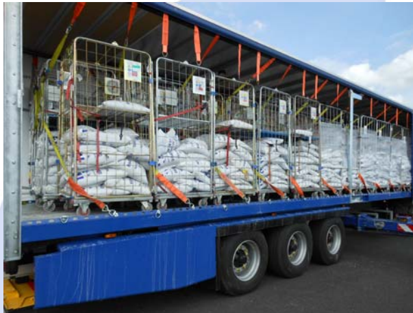
View of Diagonal Cross Strap System
